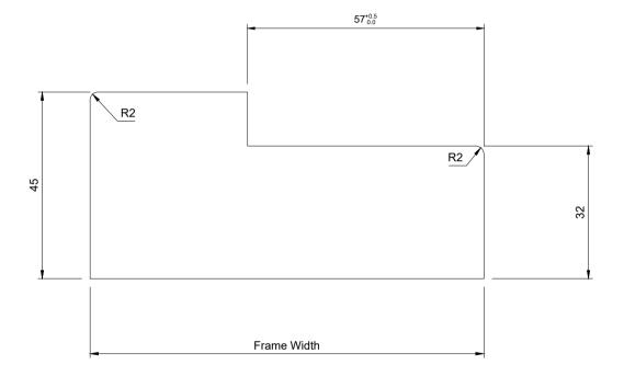
Description: Purchasing Profile Timber System 2 - 45/32 Profile - NFR - 54mm Door - Acoustic - Non Q2F
